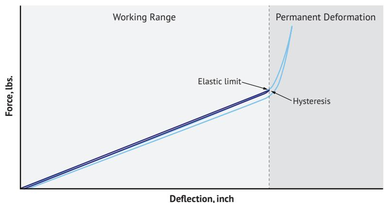
Metal bellows have negligible hysteresis as long as you keep deflection beneath the elastic limit as shown by the dark blue line. Above the elastic limit, there's permanent deformation and more significant hysteresis as indicated by light blue line.
